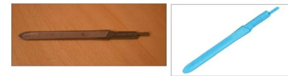
Figs. 1 and 2 – These show the original scalpel to be scanned and its stereo lithography format file.
