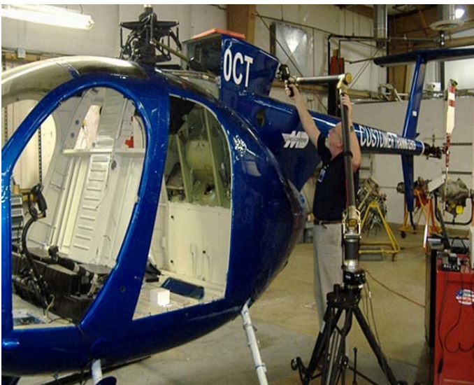
Scanning (top) rendered a complete 3D digital twin of the scanned helicopter (bottom).
