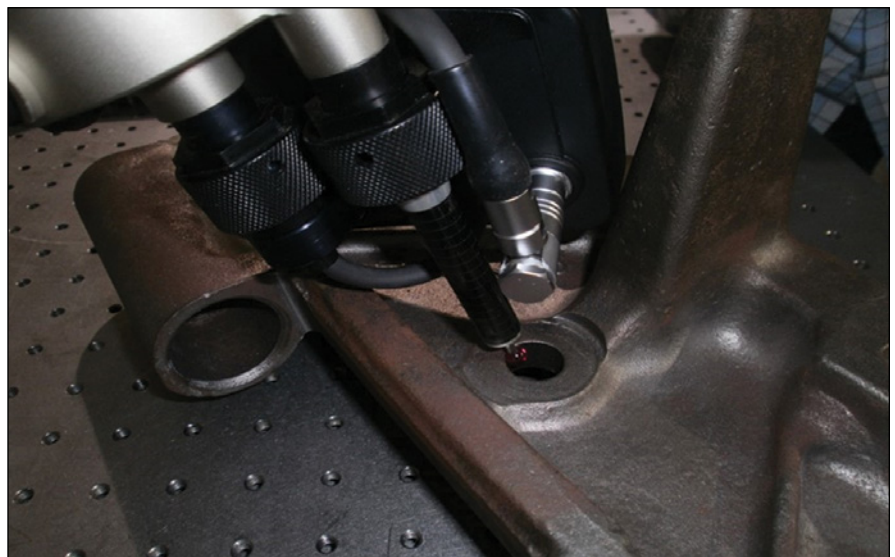
CMM probe being utilized to characterize geometric features of the interior surfaces of the pictured assembly. (Image: NVision)
